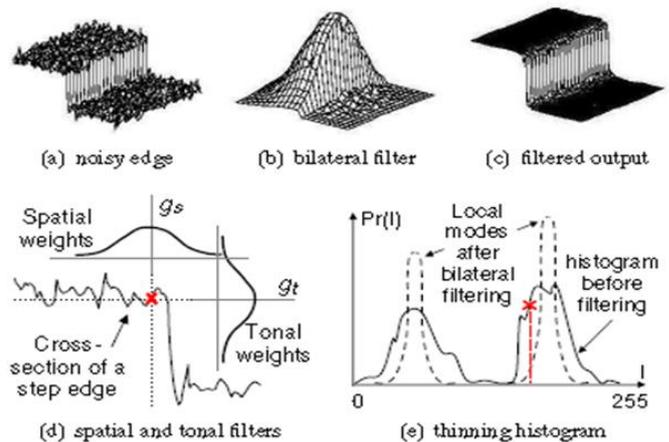
Figure 4. Bilateral filtering as a mode seeking process
