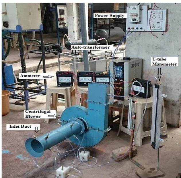
**Figure 3.** Actual test setup
