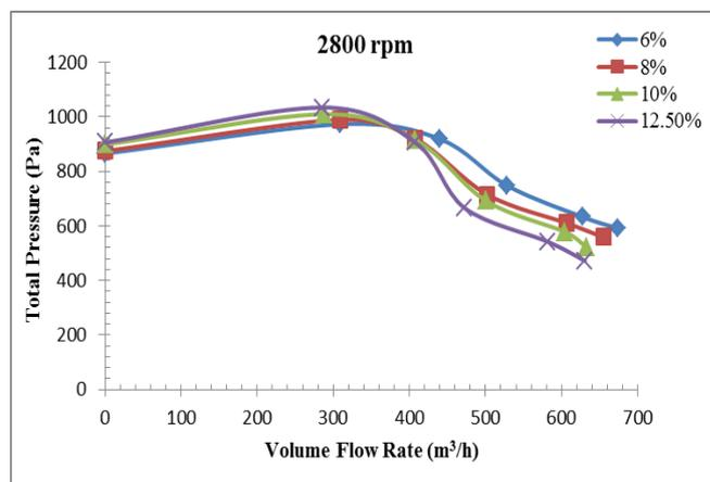
**Figure 4.** Effect of volume flow rate on total pressure at 2800 rpm
