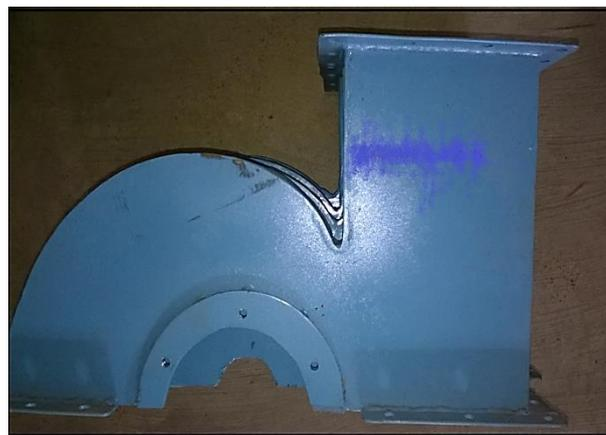
**Figure 2.** Casings with Different Volute Tongue Clearances
