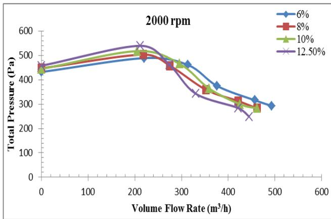
**Figure 6.** Effect of volume flow rate on total pressure at 2000 rpm
