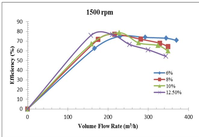
**Figure 11.** Effect of volume flow rate on efficiency at 1500 rpm
