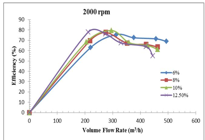
**Figure 10.** Effect of volume flow rate on efficiency at 2000 rpm
