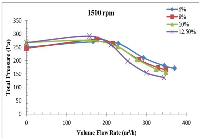
**Figure 7.** Effect of volume flow rate on total pressure at 1500 rpm
