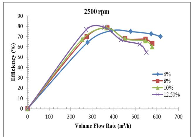
**Figure 9.** Effect of volume flow rate on efficiency at 2500 rpm
