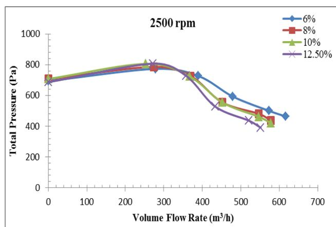
**Figure 5.** Effect of volume flow rate on total pressure at 2500 rpm
