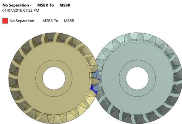
Figure 5: Detailed view of gear tooth contact between two gears.
