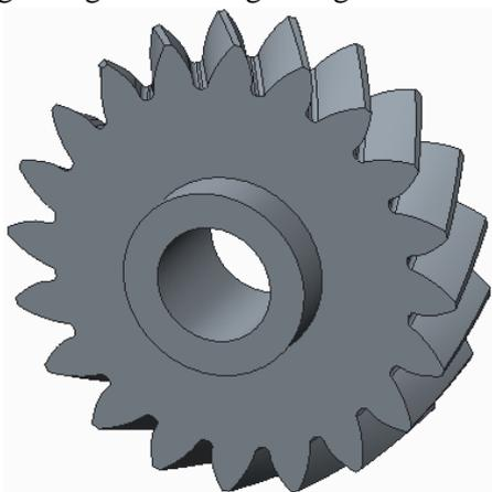
**Figure 1:** Model of asymmetric helical gear.
