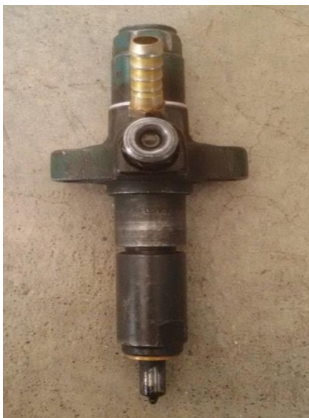
Figure 2. Bosch fuel injector
