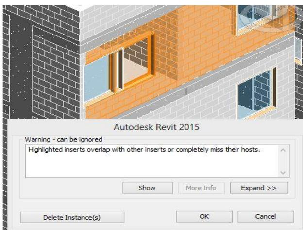
**Figure 2.** Interface check (example clashed elements)
