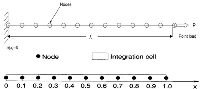
Figure 3. 1-D bars with node and integration cell
