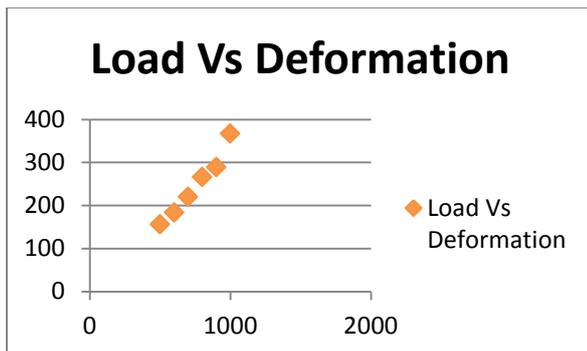
**Graph 3:** Load Vs. Deformation for New Spring
