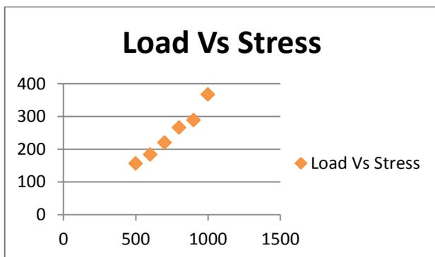
**Graph 4:** Load Vs. Stress for New Spring
