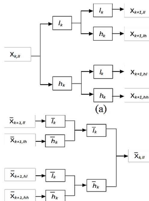
Figure 2: one level filter bank implementation of DWT. (a)Forward Pass (b) Backward Pass
