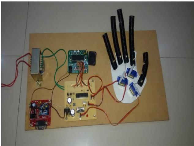
**Figure 7.** Receiver Section
