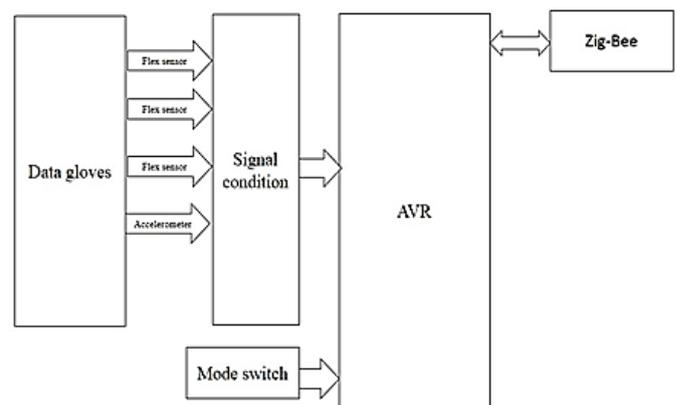
**Figure 1.** Block diagram of transmitter section
