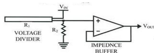
Figure 4. Basic Flex Sensor circuit [21]
