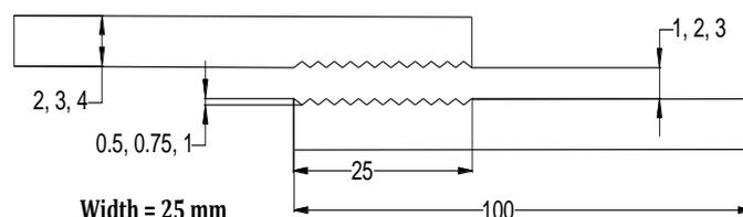
Figure 1. Joint geometry (All dimensions are in mm)
