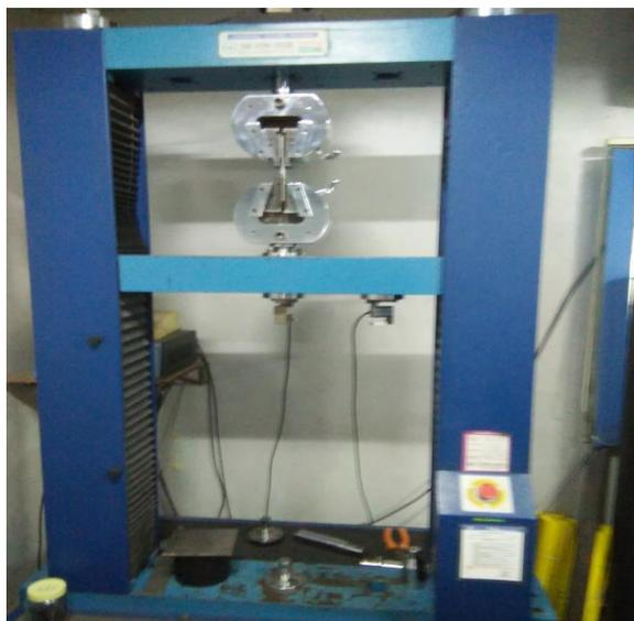
**Figure 3.** Universal testing machine with test piece
