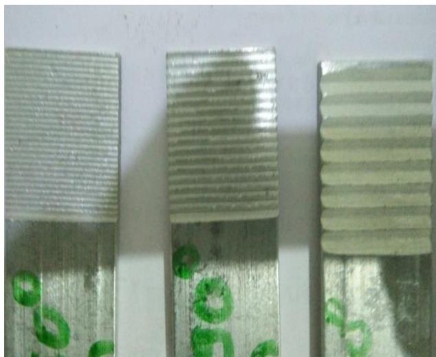
Figure 2. Surface prepared with variable pattern
