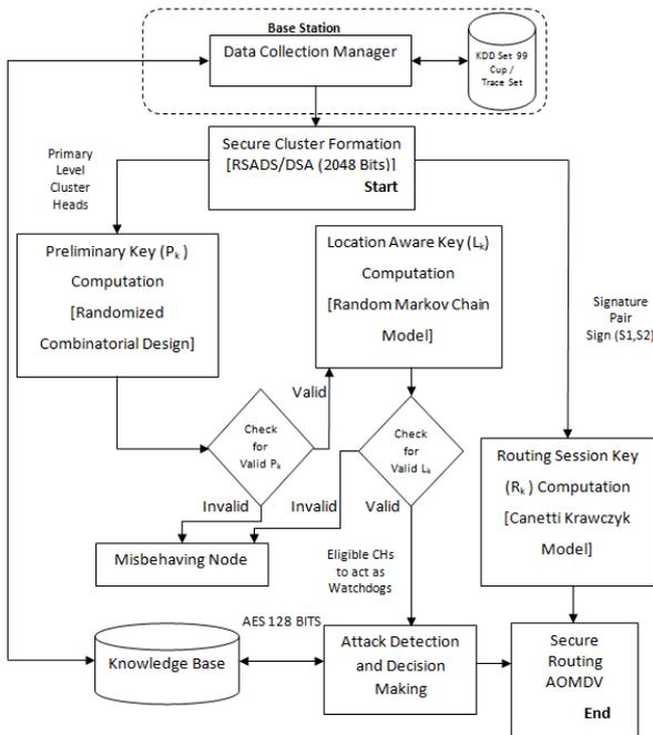
**Figure 3.2** – Secure key management based watchdog selection scheme
