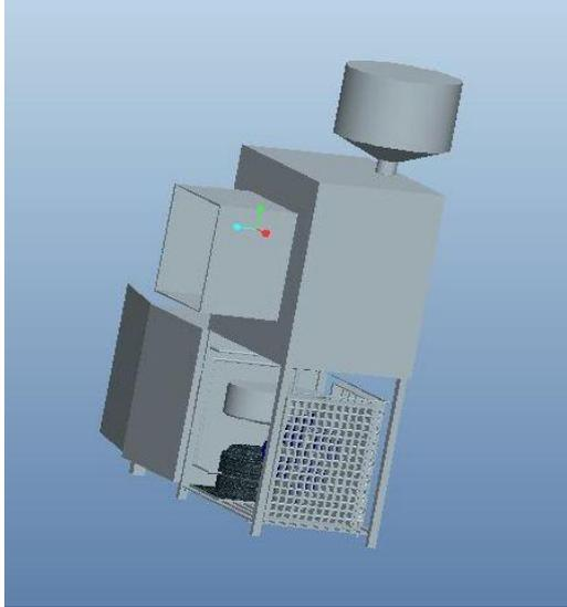
**Figure 1.** CAD Model of Refrigeration cum Air Conditioner and Water Cooler unit
