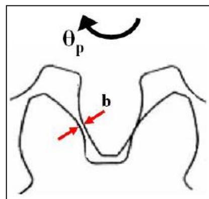
**Figure 1.** Gears in meshing vibrate due to backlash (b)<sup>[6]</sup>
