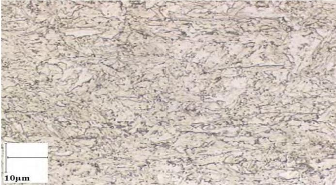
**Figure 2.8 :** Photomicrograph of CP 800/1000 hot rolled steel.
