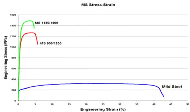
**Figure 2.7 :** Engineering stress/ strain curves for various type of MS steel grades
