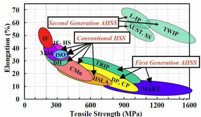
**Figure 2.** Relationship between tensile strength and total elongation (50.8mm gauge length) for various types of steel (r/t) for various AHSS (International Iron and Steel Institute, 2006)
