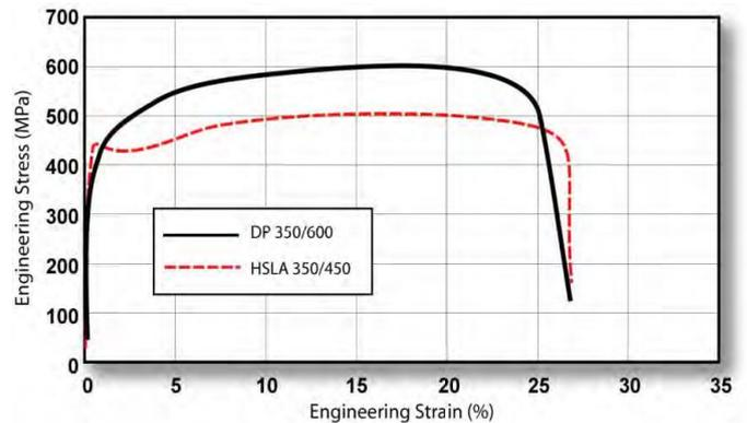
**Figure 2.3.** The DP 350/600 with higher TS than the HSLA 350/450K
