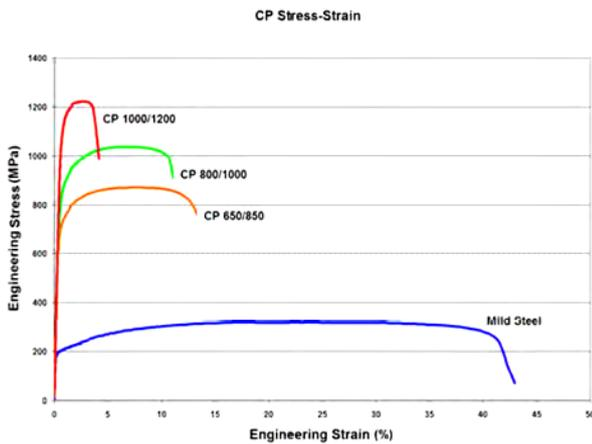
**Figure 2.9 :** Engineering stress-strain curves for a series of CP steel grades. V-1 Sheet thickness: CP650/850 = 1.5mm, CP 800/1000 = 0.8mm, CP 1000/1200 = 1.0mm, and Mild Steel = approx. 1.9mm (International Iron and Steel Institute, 2006).
