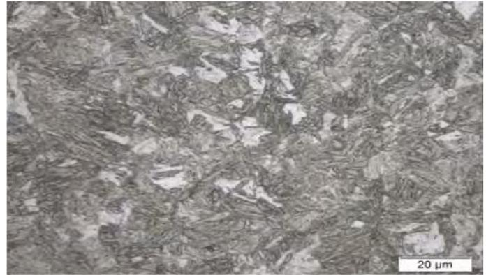
**Figure 2.6:** Microstructure for MS 950/1200
