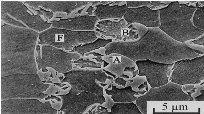
**Figure 2.5 :** A typical multiphase microstructure of a modern TRIP-assisted steel, with allotriomorphic ferrite (F), carbide-free bainite (B) and retained austenite (A).
