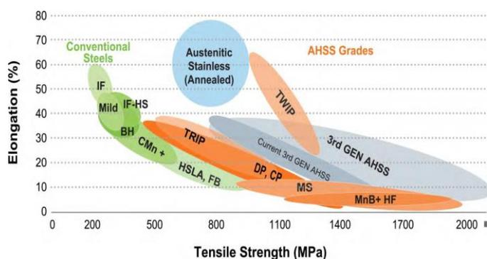
**Figure 1.** Global formability diagram, illustrating the range of properties available from today’s AHSS grades (WorldAutoSteel, 2014).
