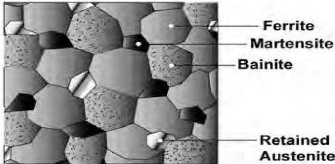
**Figure 2.4 :** Bainite and retained austenite are additional phases in TRIP steels
