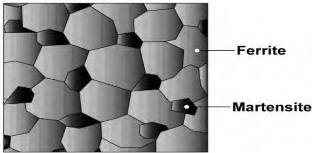
**Figure 2.1:** Schematic shows islands of martensite in a matrix of ferrite
