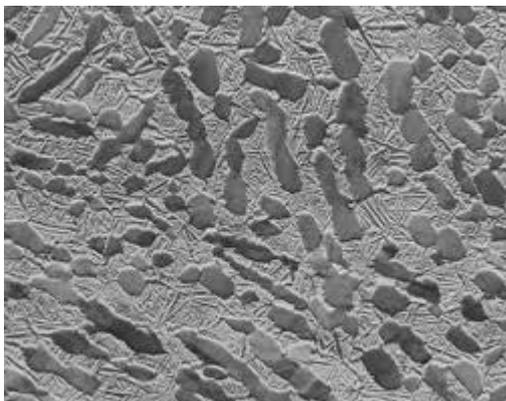
**Figure 2.2.** Photomicrograph of DP steel
