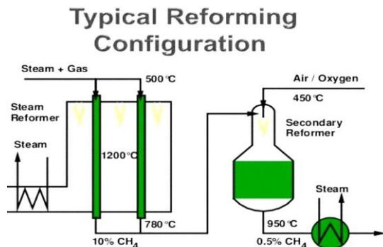
**Figure 1.** Typical Reforming Configuration.
