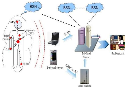
**Figure 2:** Diagram of Body Sensor Network
