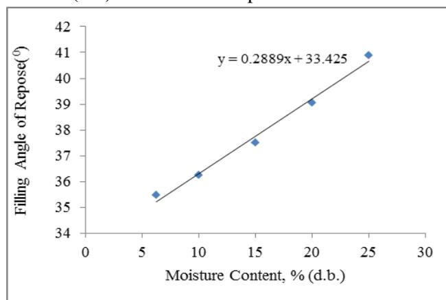
Fig. 9 Effect of moisture content on filling angle of repose of shea kernels
