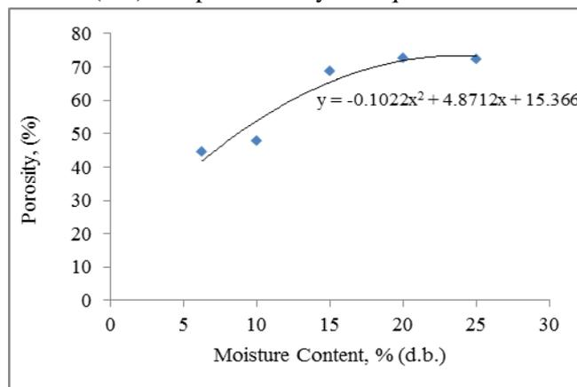
Fig. 8 Effect of moisture content on shea kernel's porosity
