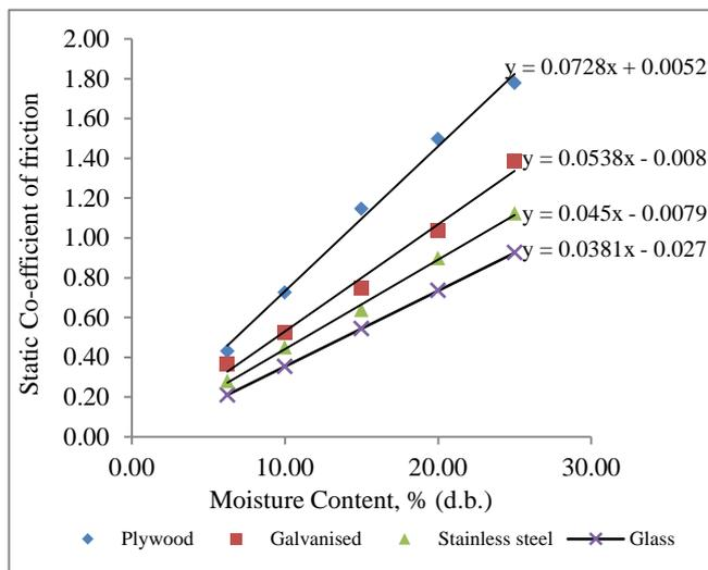
Fig. 10 Effect of moisture content on static co-efficient of friction of shea kernel
