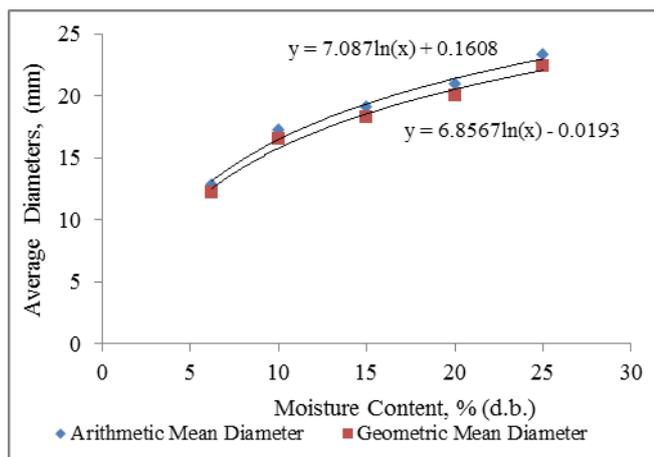
**Fig. 2.** Effect of moisture content on average diameters of shea kernel
