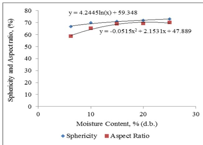
**Fig. 5** Effect of moisture content on sphericity and aspect ratio of shea kernel
