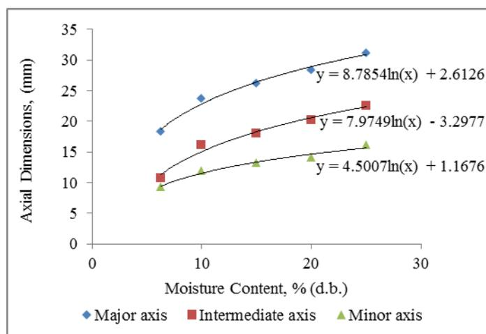
Fig. 1 Effect of moisture content on triaxial dimensions of shea kernel
