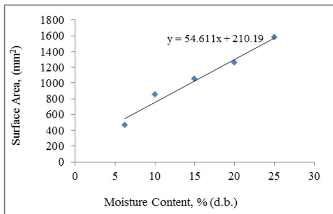
**Fig. 3** Effect of moisture content on surface area of shea kernel
