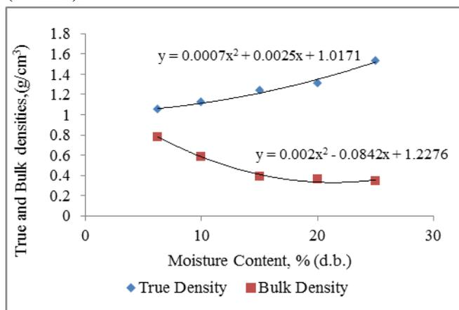
Fig. 7 Effect of moisture content on true and bulk density of shea kernel
