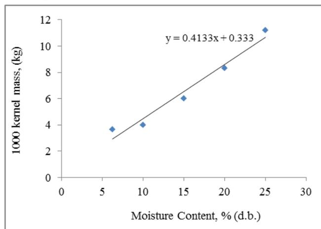
**Fig. 6** Effect of moisture content on 1000 kernel mass of shea kernel
