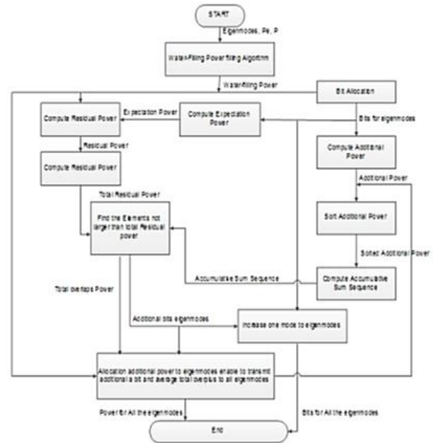
Figure 5. Flow chart of adaptive power control algorithm
