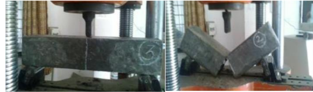
Figure 2.(a)Test Specimen (Beam) (b) Flexural strength with point loading
