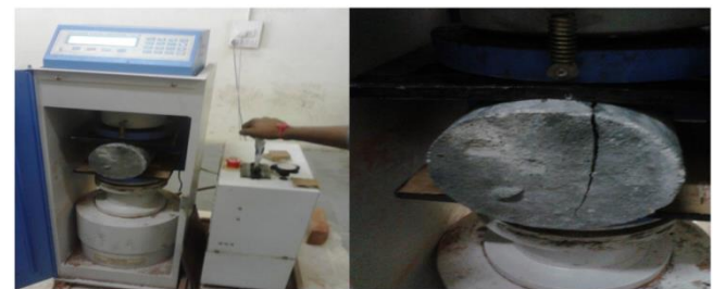
Figure 3.Compression testing machine/ Applied load on cylinder / Failure of Cylinder
