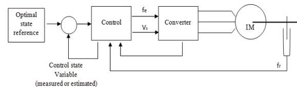
**Figure b.** Block Diagram of Simple State Control
