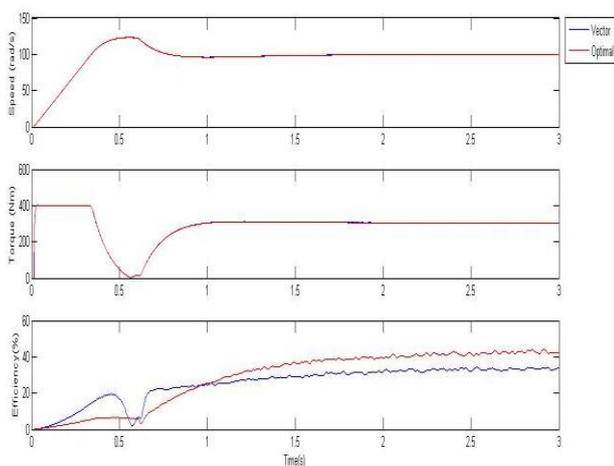
**Figure h.** Speed, Torque and Efficiency performance at rated load torque (300N-m) at 100 rad/sec speed
