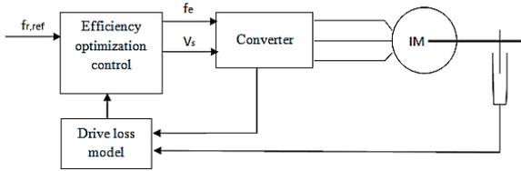
**Figure c.** Block Diagram of Model Based Control
