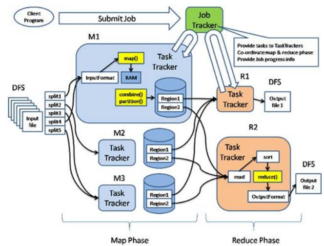
**Figure 4.** MapReduce Procedure
