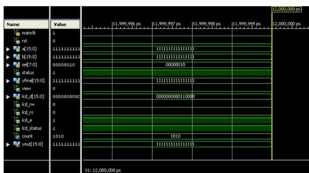
Figure 12. Waveform of OR operation.
