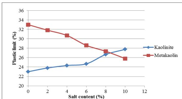
Fig. 4: Variation of Plastic limit with NaCl
