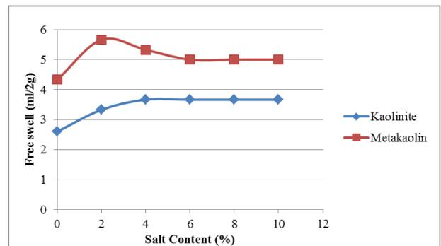
Fig. 7: Variation of Free swell index with NaCl
