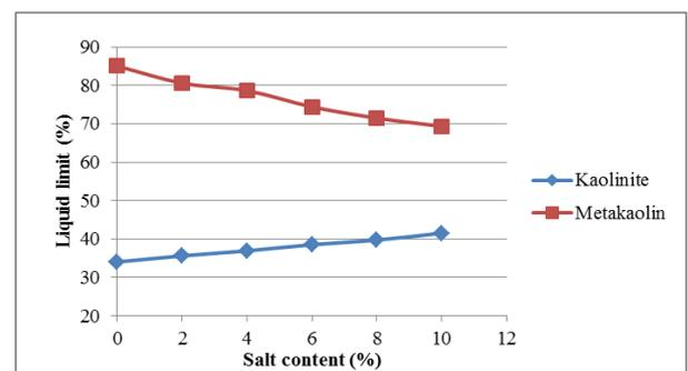
Fig. 3: Variation of Liquid limit with CaCl<sub>2</sub>
