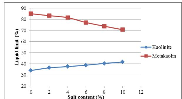
Fig. 1: Variation of Liquid limit with NaCl
