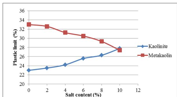
Fig. 5: Variation of Plastic limit with MgCl<sub>2</sub>
