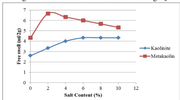
Fig. 9: Variation of Free swell index with CaCl<sub>2</sub>
