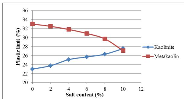
Fig. 6: Variation of Plastic limit with CaCl<sub>2</sub>
