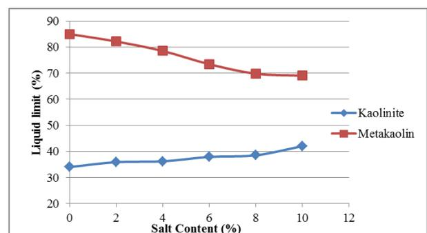
Fig. 2: Variation of Liquid limit with MgCl<sub>2</sub>
