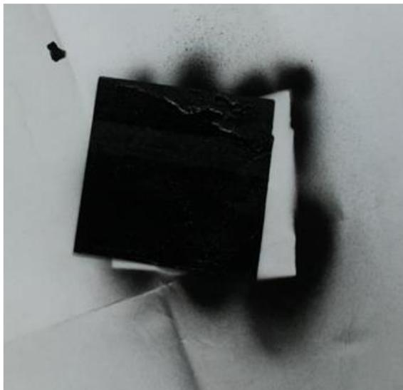
**Figure 1.** Carbon paper coated with the Catalyst Slurry.
