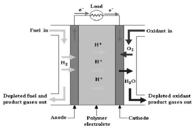
**Figure 1.** Principle of PEM fuel cell
