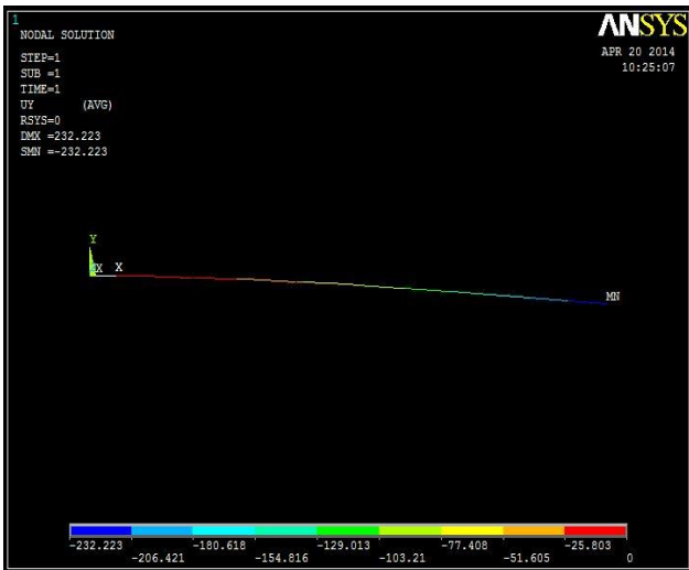
Figure 6. Deflection of cantilever beam (T Cross-section)
