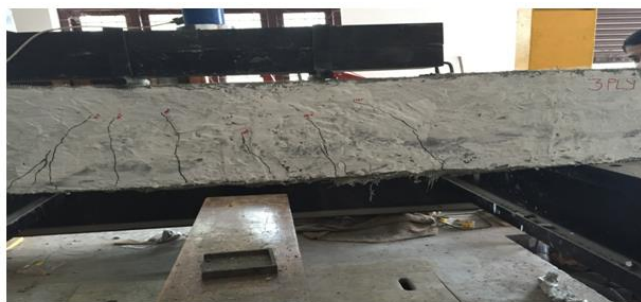
Figure 7. Testing of 3ply FRCM beam
