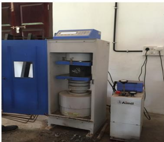
Figure 1. Testing of Compressive strength of Concrete
