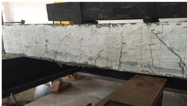
Figure 6. Testing of 1ply FRCM beam
