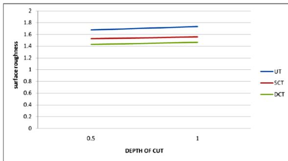
**Figure 5.7** - Effect of depth of cut on surface roughness for nose radius 0.4 mm
