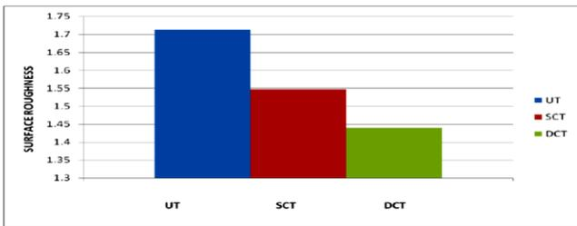
**Figure 5.1** Comparison of surface roughness by UT, SCT and DCT for nose radius 0.4 mm
