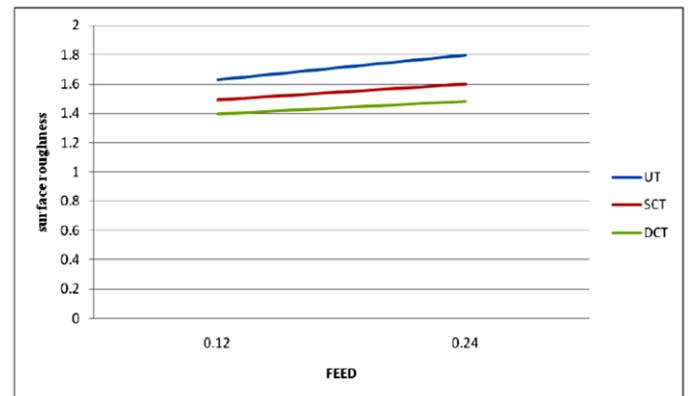
**Figure 5.8** - Effect of feed on surface roughness for nose radius 0.4 mm
