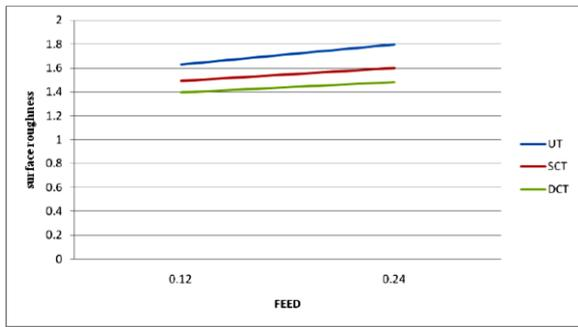
**Figure 5.6** - Effect of feed on surface roughness for nose radius 0.8 mm
