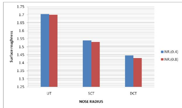
**Figure 5.9** Effect of nose radius on surface roughness
