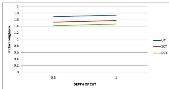
**Figure 5.8** Effect of depth of cut on surface roughness for nose radius 0.8 mm
