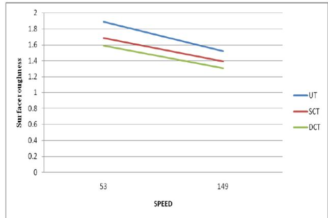
**Figure 5.4** Effect of speed on surface roughness for nose radius 0.8 mm
