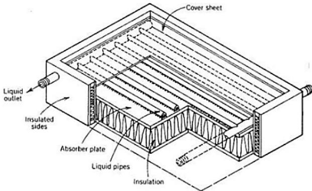
**Figure 1: Flat Plate Collector**
