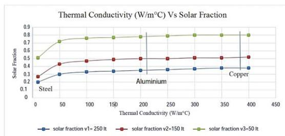
**Figure 4 :** Thermal Conductivity (W/m°C) Vs Solar Fraction
