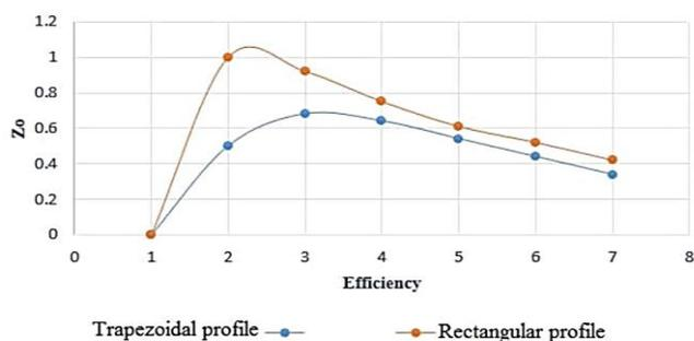
**Figure 8 :** Efficiency Vs  $Z_o$
