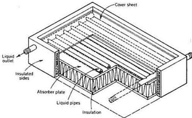
Figure 1: Flat Plate Collector
