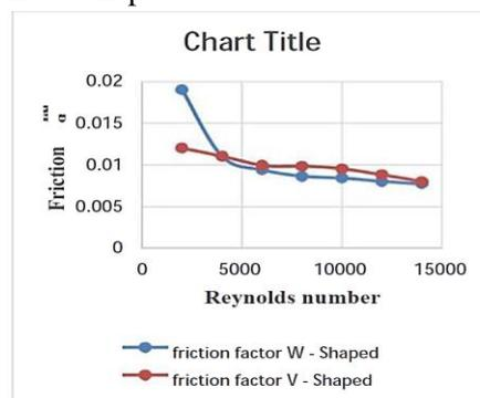
**Figure 6 :** Reynolds Number Vs Friction Factor
