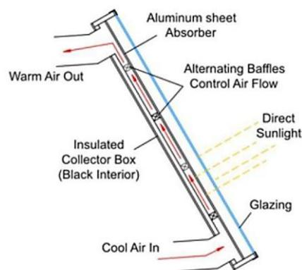
**Figure 5 :** Solar Air Heater
