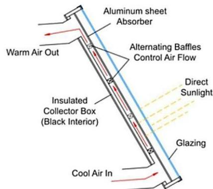
**Figure 5 :** Solar Air Heater
