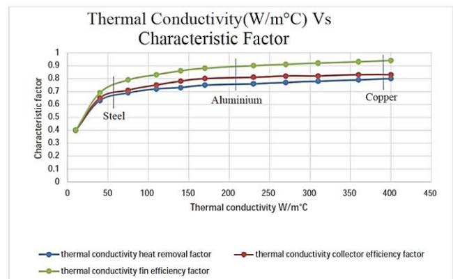
**Figure 3 : Thermal Conductivity(W/m°C) Vs Characteristic Factor**
