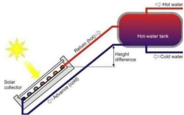
**Figure 2: Solar Water Heater**
