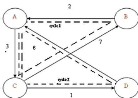
**Figure 2.** Mesh Network with P-cycles
