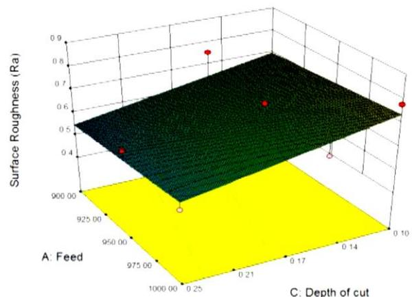
**Chart-2 (b):** Response Surface at C.S of 3500 RPM
