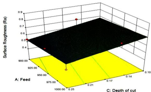
**Chart-2 (c):** Response Surface at C.S of 3900 RPM
