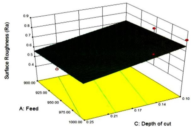
**Chart-2 (a): Response Surface at C.S of 3100 RPM**
