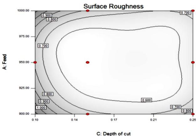
**Chart-1 (c) :** Feed & Depth of Cut at Cutting Speed of 3900 RPM
