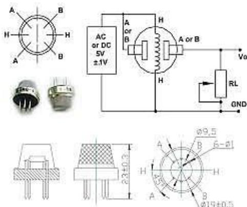
Figure 4. The MQ4 gas sensor.
