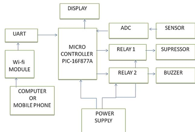
**Figure 2.** Block diagram of user interactive toxic gas suppressor system.
