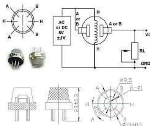
Figure 4. The MQ4 gas sensor.
