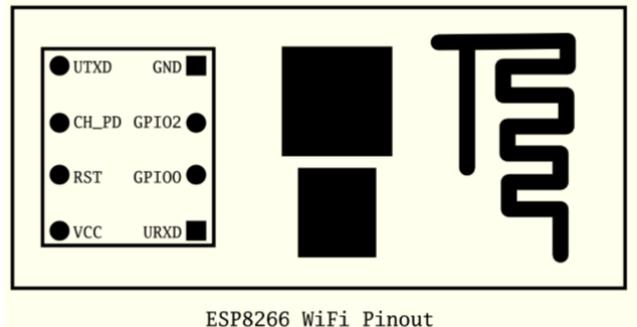
Figure 5. Pin out configuration of ESP8266
