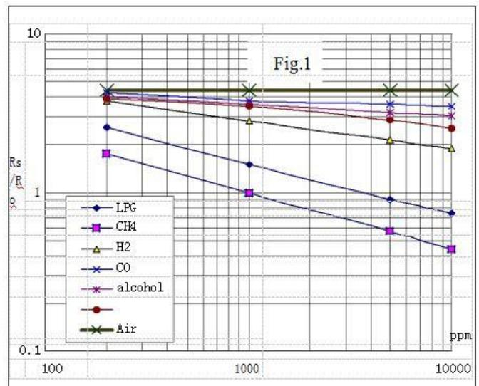
**Figure 1.** Sensitivity characteristics of various gases in MQ4 sensor.
