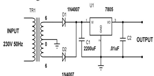
Figure 7. Power supply circuit diagram
