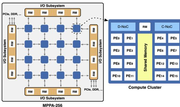
**Figure 8** : Kalray MPPA-256 Bostan processor Architecture overview
