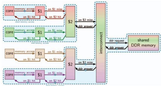
**Figure 2 :** Multicore architecture with cache coherent memory.
