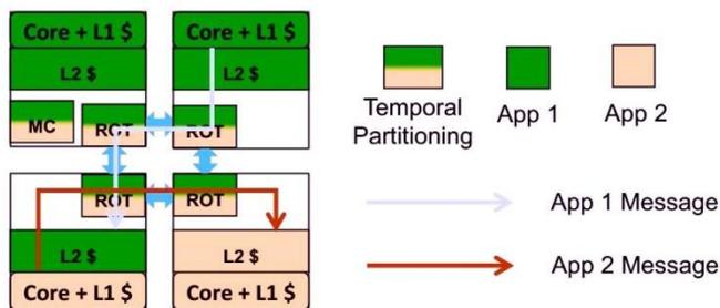
**Figure 1:** Interference Channels in Multicore Platform
