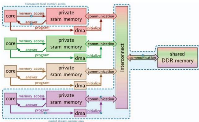
**Figure 3:** Multicore architecture with local memories
