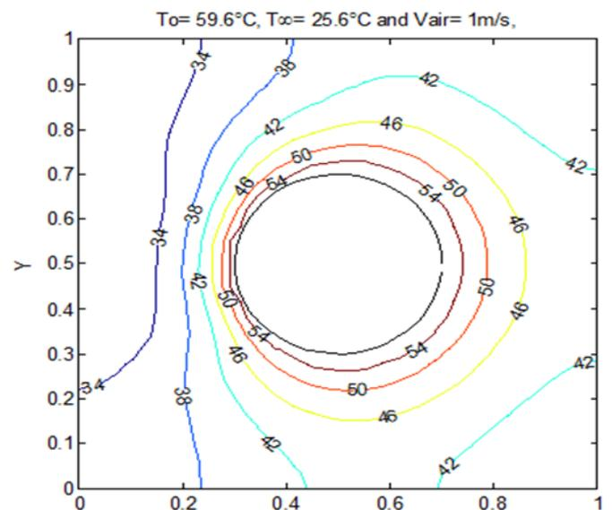
**Figure 4.** Variation of fin temperature over fin surface for 1m/sec velocity for  $\Delta T=33^\circ\text{C}$
