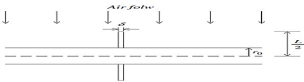
**Figure 1.** schematic diagram of one-tube plate fin heat exchanger [chen 2006]
