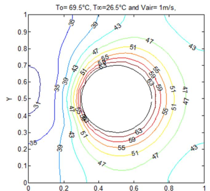
**Figure 5.** Variation of fin temperature over fin surface for 1m/sec velocity for  $\Delta T=43^\circ\text{C}$
