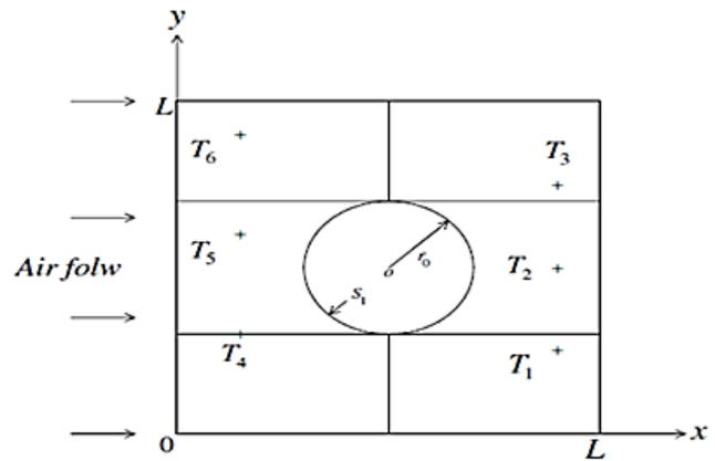
**Figure 2.** physical geometry of two-dimensional plate fin with a circular tube
