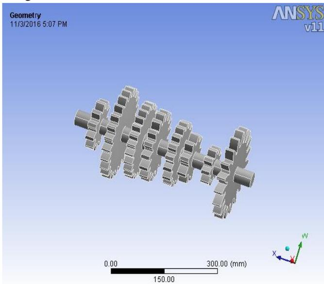
Figure 3. Geometric model of counter shaft
