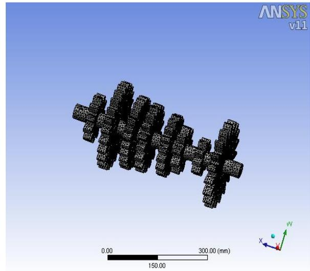
Figure 4. Meshing the Shaft
