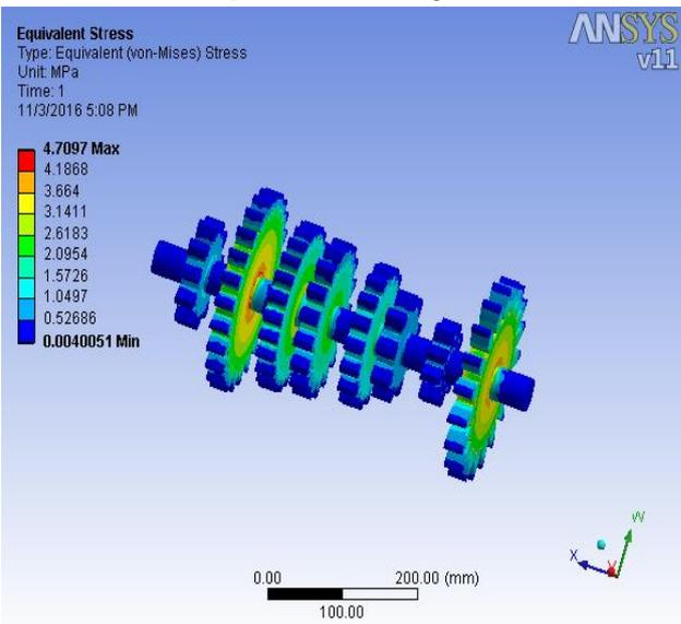
Figure 5. Equivalent stress
