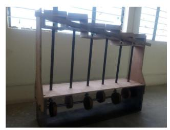
**Figure 3.4.** Cam operated conveyor assembly
