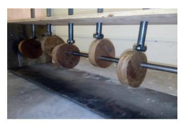
Figure 3.1 Shaft and cams assembly
