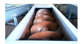
Figure 1.3 Screw conveyor
