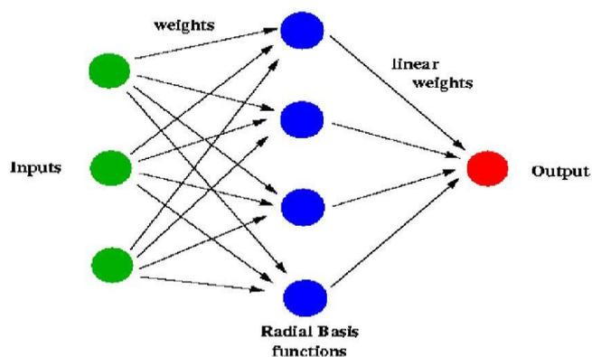
Figure 4. Radial basis function
