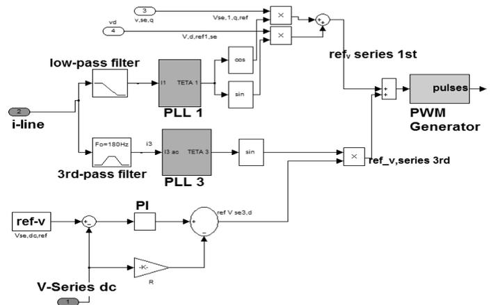
**Figure 5. Block diagram of series control structure in Matlab/Simulink**
