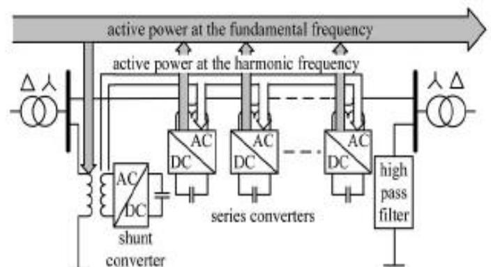
Figure 2. Active power exchange between DPFC convertes
