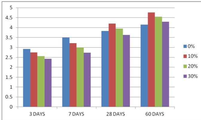
**Figure 3.** Variation of 28 Days Split Tensile Strength M20 Grade
