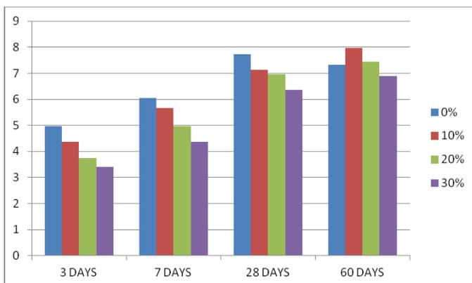
**Figure 5.** Variation of 28 Days Flexural Strength M20 Grade
