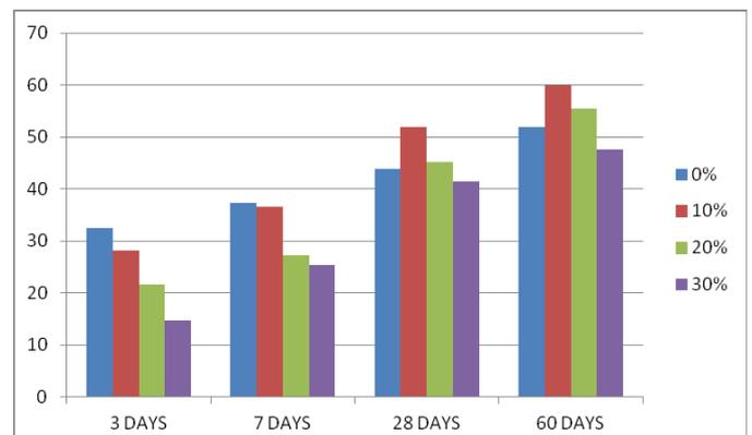
Figure 2. Variation of 28 Days Compressive Strength M30 Grade
