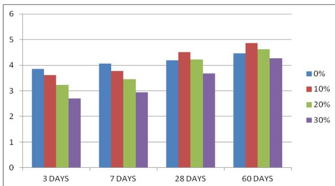
**Figure 4.** Variation of 28 Days Split Tensile Strength M30 Grade
