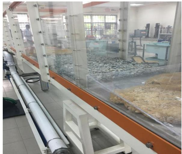
**Figure 2 :** showing Gravel bed in the flume
