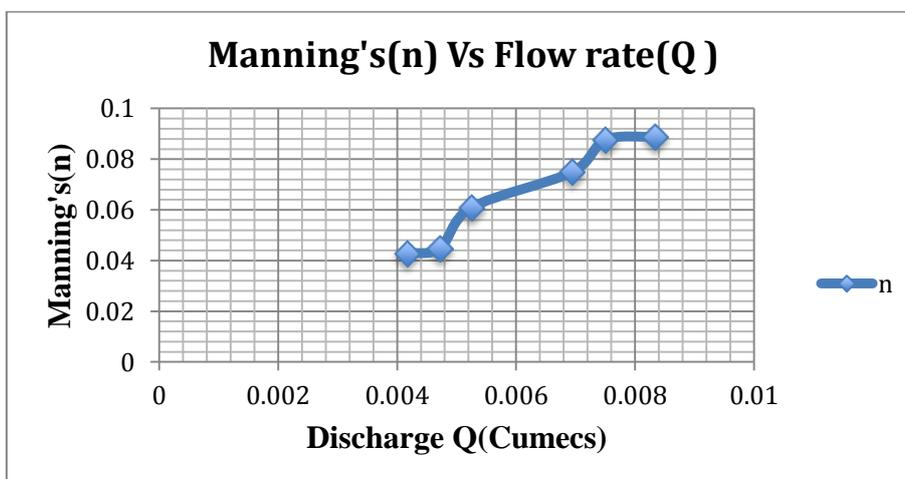
Figure 6 : Graph of Mannings (n) against Discharge (Q) of water using rectangular weir
