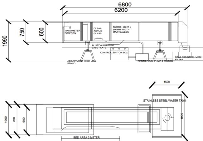
Figure 4 : Schematic Diagram Of Experimental Setup
