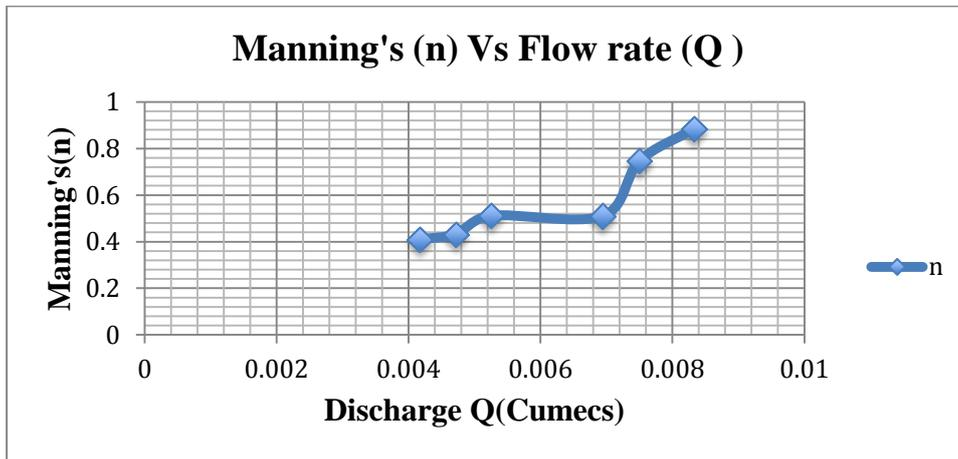
Figure 4.5 Graph of Mannings (n) against Discharge (Q) of water using rectangular weir
