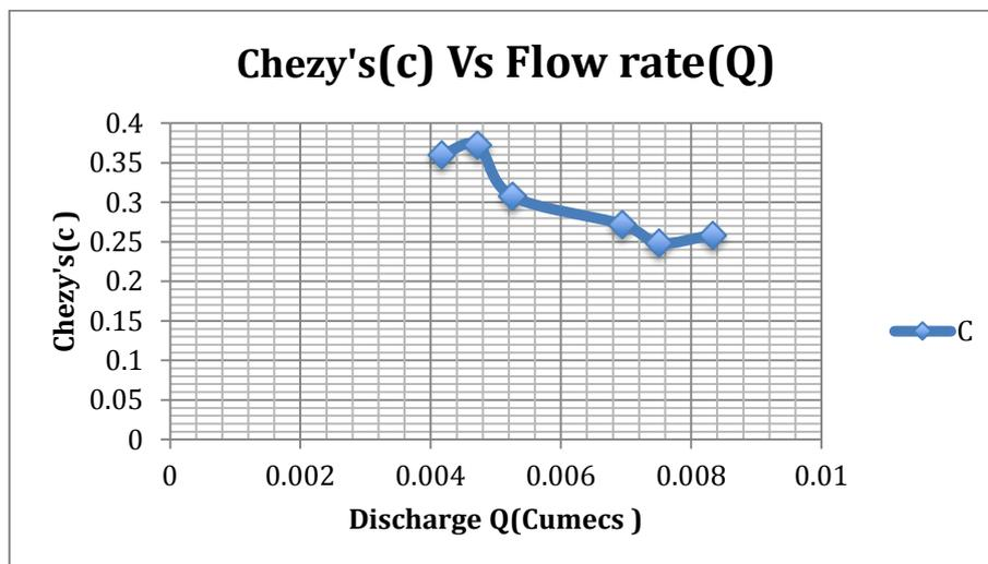
Figure 5: Graph of Chezy's (c) against Discharge (Q) of water using rectangular weir
