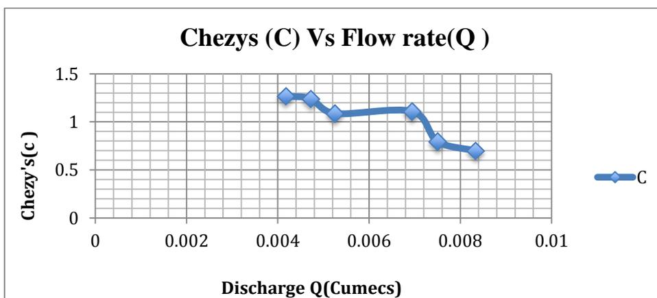
Figure 4.6 Graph of Chezy's (c) against Discharge (Q) of water using rectangular weir
