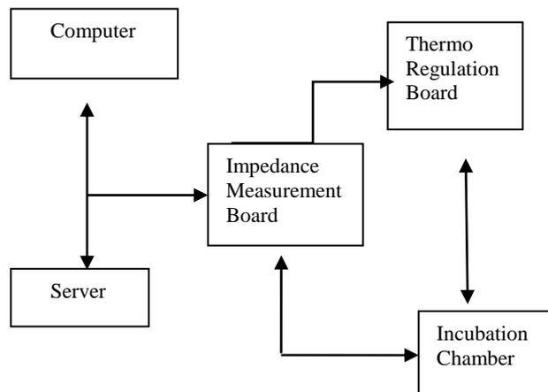
Impedance measure board enables the thermoregulation board after receiving the start signal. Then thermoregulation board waits for 30 minutes for the SUT temperature to stabilize. Then, it measures electrical parameters of the SUT at time intervals of 5 minutes. When the variation is above 5% when compared to baseline value, it calculates the detect time.
