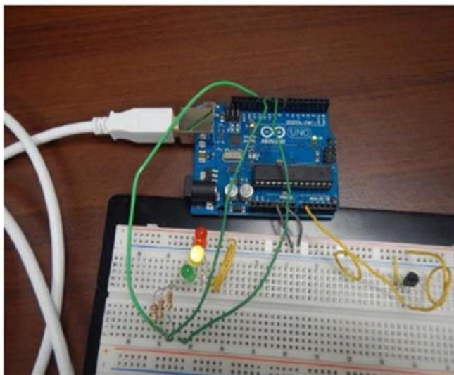
Figure 2. Microcontroller board with temperature sensor
