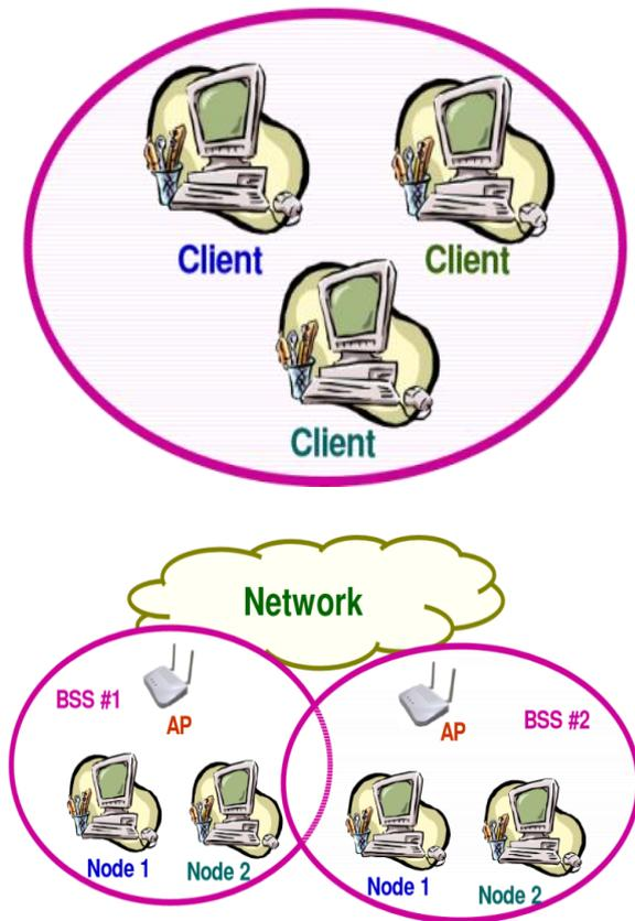
**Figure 1-1.** Ad Hoc and Infrastructure Network Topologies
