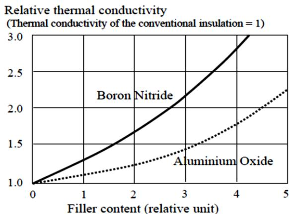
**Figure 2.** Thermal conductivity of insulation as a function of filler and content
