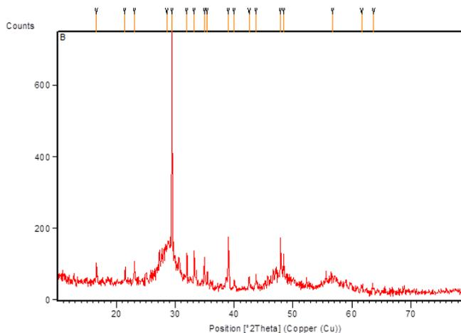
**Figure 2:** XRD Pattern of Sample B
