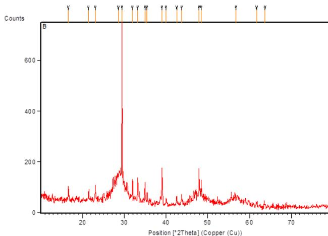
**Figure 2:** XRD Pattern of Sample B
