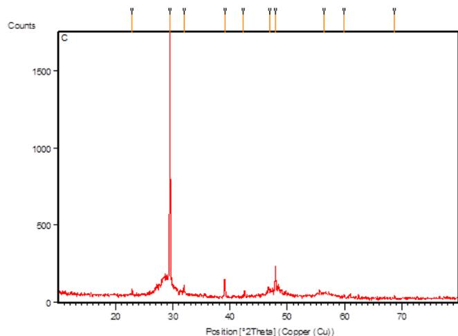
**Figure 1:** XRD Pattern of Sample A
