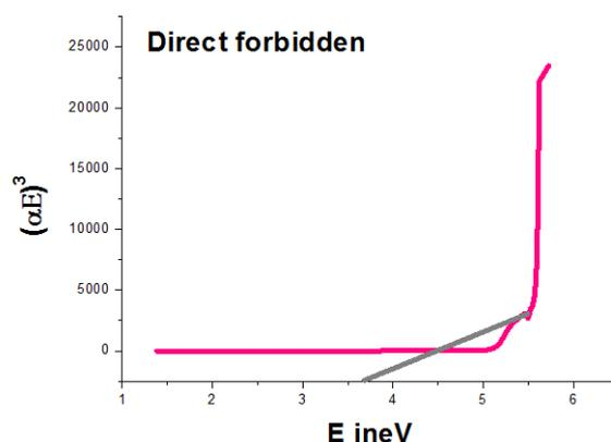
**Figure 6:** Direct Bandgap for Sample C
