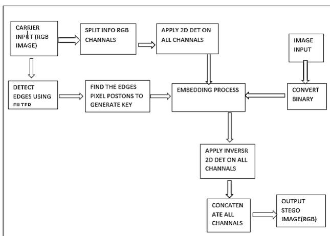
Figure 4. Block Diagram of Encoding Process
