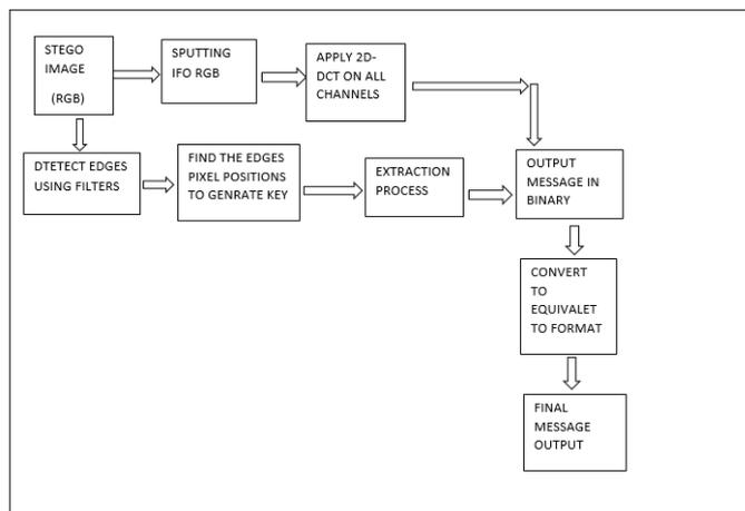
**Figure 3.** Block Diagram of Decoding Process
