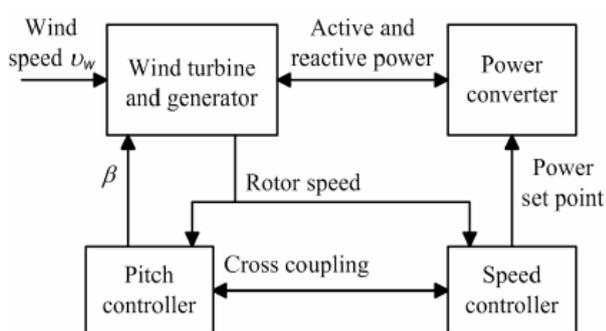
**Figure 1.** Block diagram of variable-speed wind turbine
