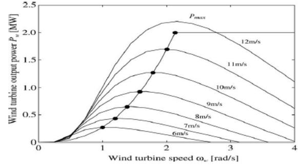
Figure 3. output characteristics of wind turbine
