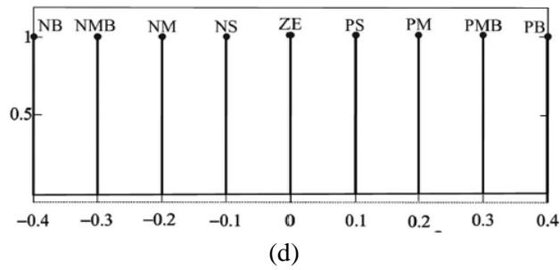
**Figure 5.** Membership functions of FLC for (a) error of generator output power. (b) Variation of power error. (c) Rotational speed. (d) Pitch angle reference
