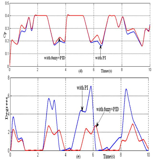
**Figure 9.** Simulation results for PI controller, and proposed hybrid FLC at the mean wind speed of 12 m/s. (a) Generator powers. (b) Rotor speeds. (c) Mechanical torques. (d) Power conversion coefficients. (e) Pitch angles.
