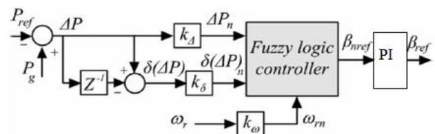
**Figure 4.** Block diagram of pitch control system using Hybrid FLC
