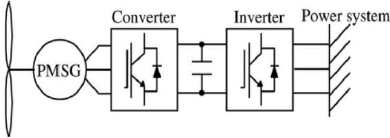
Figure 2. Gearless WECS using PMSG.
