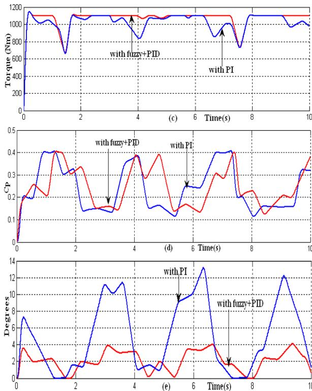
**Figure 8.** Simulation results for PI controller, and proposed hybrid FLC at the mean wind speed of 14 m/s. (1)Wind speeds. (a) Generator powers. (b) Rotor speeds. (c) Mechanical torques. (d) Power conversion coefficients. (e) Pitch angles.
