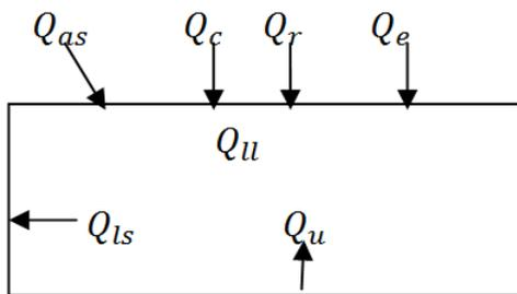
Figure 3 : Heat balance in the upper zone
