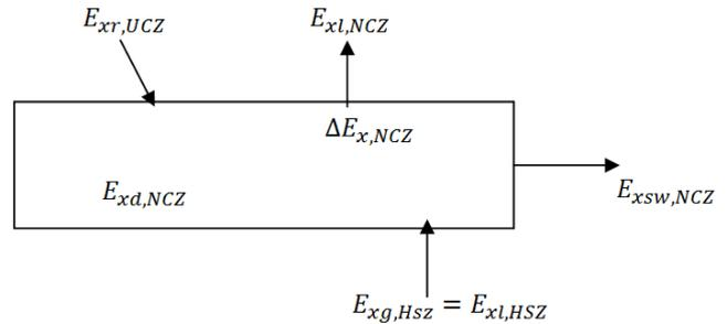
**Figure 6 :** Energy and Exergy flows in the NCZ of Solar Pond
