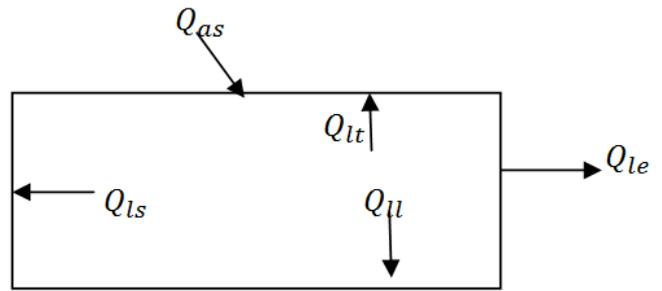
Figure 4 : Heat balance in the storage zone
