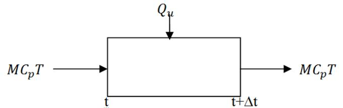
Figure 2 : Heat balance of volume
