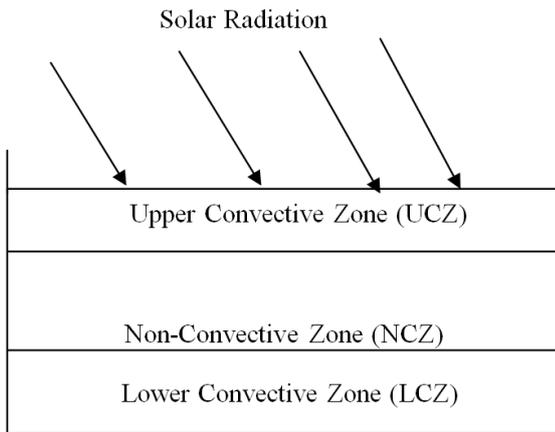
Figure 1 : Schematic view of a solar pond
