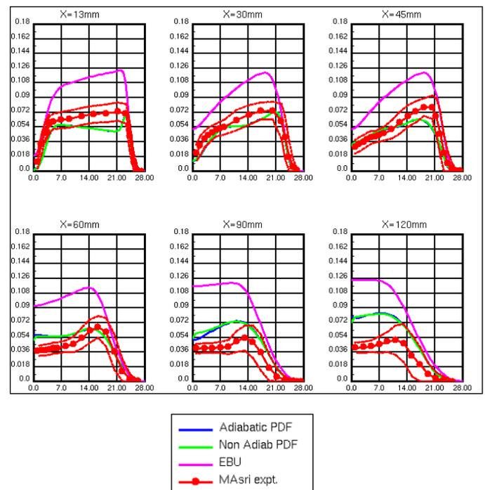
**Figure 5:** Carbon dioxide CO<sub>2</sub> predictions for PPDF model versus test data.
