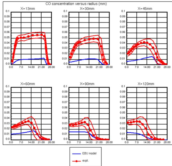
**Figure 2:** Carbon monoxide CO mass concentration for the EBU model
