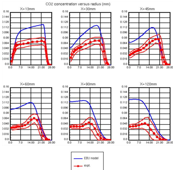
**Figure 3:** Carbon dioxide CO<sub>2</sub> mass concentration for the EBU model
