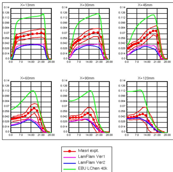
**Figure 7 :** Carbon dioxide CO<sub>2</sub> predictions for Laminar flamelet model versus test data.
