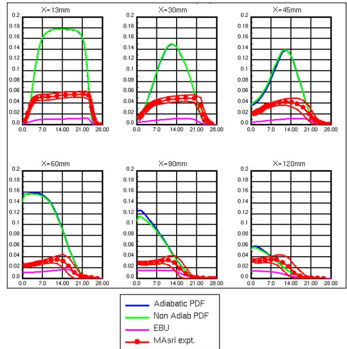
**Figure 4:** Carbon monoxide CO predictions for PPDF model versus test data.
