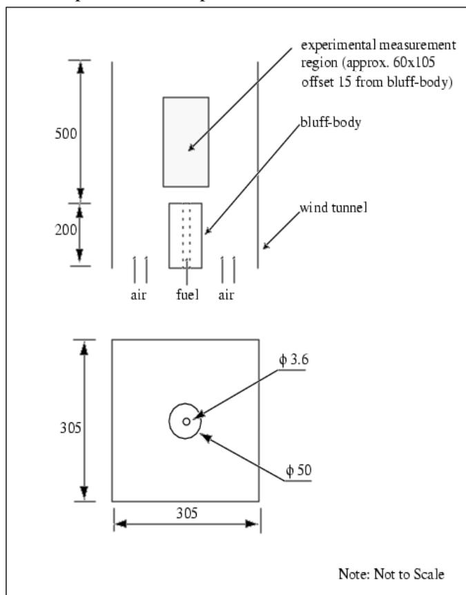
**Figure 1:** Schematic of the Masri Bluff body burner. (in mm)
