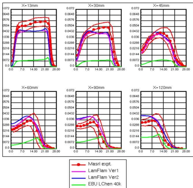
**Figure 6 :** Carbon monoxide CO predictions for Laminar flamelet model versus test data.
