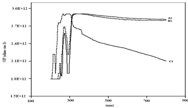
**Figure 22 :** Optical conductivity spectra of samples, shapes: (a) pure PVC, (b) PVC doped 10% ZnO, and (c) PVC doped 15% ZnO. Energies of CO<sub>2</sub> Laser: 400 mJ
