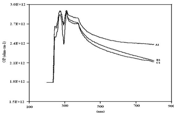
**Figure 33 :** Optical conductivity spectra of samples, shapes: (a) pure PVC, (b) PVC doped 10% ZnO, and (c) PVC doped 15% ZnO. Energies of CO<sub>2</sub> Laser: 500 mJ
