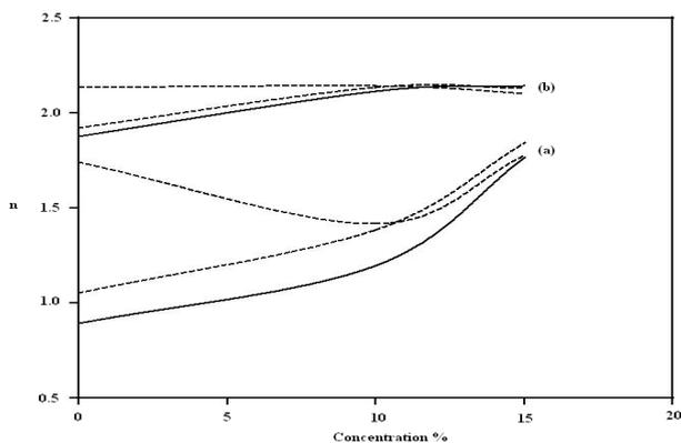
**Figure 10 :** The variation of refractive index versus different concentrations of ZnO in PVC: (A) 300 mJ, (B) 400 mJ, and (C) 500 mJ. At specific wavelengths (a) 300 nm, (b) 500 nm.
