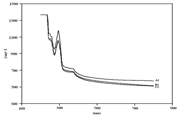
**Figure 8 :** Absorption coefficient spectra of samples, shapes: (a) pure PVC, (b) PVC doped 10% ZnO, and (c) PVC doped 15% ZnO. Energies of CO<sub>2</sub> Laser: 400 mJ
