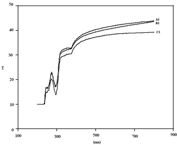
**Figure 2 :** Transmission spectra of samples, shapes: (a) pure PVC, (b) PVC doped 10% ZnO, and (c) PVC doped 15% ZnO. Energies of CO<sub>2</sub> Laser: 400 mJ
