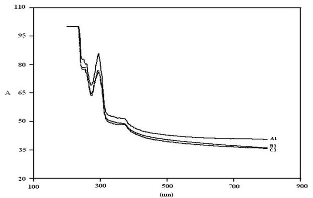
**Figure 4 :** Absorption spectra of samples, shapes: (a) pure PVC, (b) PVC doped 10% ZnO, and (c) PVC doped 15% ZnO. Energies of CO<sub>2</sub> Laser: 300 mJ
