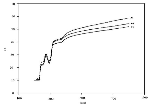
**Figure 3 :** Transmission spectra of samples, shapes: (a) pure PVC, (b) PVC doped 10% ZnO, and (c) PVC doped 15% ZnO. Energies of CO<sub>2</sub> Laser: 500 mJ
