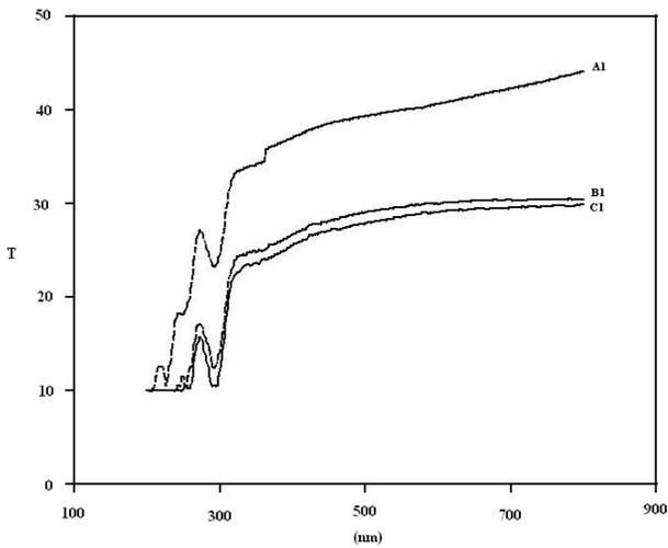
**Figure 1 :** Transmission spectra of samples, shapes: (a) pure PVC, (b) PVC doped 10% ZnO, and (c) PVC doped 15% ZnO. Energies of CO<sub>2</sub> Laser: (A) 300 mJ
