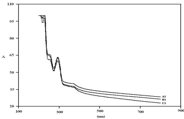
**Figure 5 :** Absorption spectra of samples, shapes: (a) pure PVC, (b) PVC doped 10% ZnO, and (c) PVC doped 15% ZnO. Energies of CO<sub>2</sub> Laser: 400 mJ
