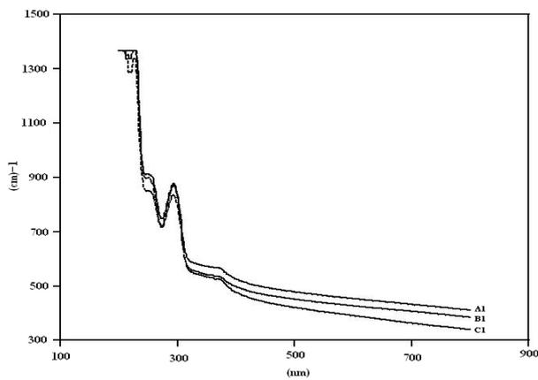
**Figure 9 :** Absorption coefficient spectra of samples, shapes: (a) pure PVC, (b) PVC doped 10% ZnO, and (c) PVC doped 15% ZnO. Energies of CO<sub>2</sub> Laser: 500 mJ
