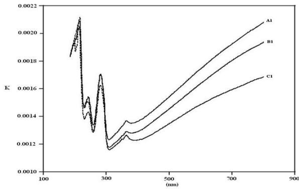
**Figure 11 :** Optical conductivity spectra of samples, shapes: (a) pure PVC, (b) PVC doped 10% ZnO, and (c) PVC doped 15% ZnO. Energies of CO<sub>2</sub> Laser: 300 mJ
