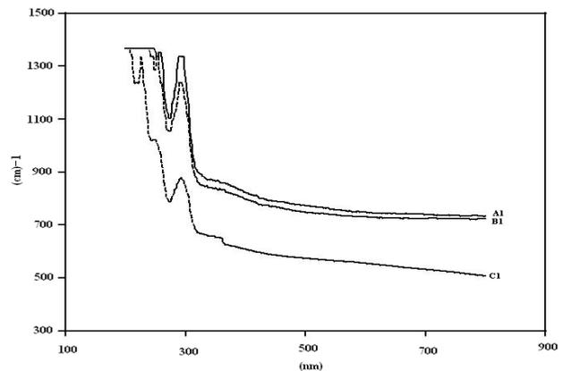
**Figure 7 :** Absorption coefficient spectra of samples, shapes: (a) pure PVC, (b) PVC doped 10% ZnO, and (c) PVC doped 15% ZnO. Energies of CO<sub>2</sub> Laser: 300 mJ
