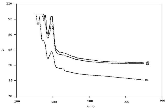
**Figure 6 :** Absorption spectra of samples, shapes: (a) pure PVC, (b) PVC doped 10% ZnO, and (c) PVC doped 15% ZnO. Energies of CO<sub>2</sub> Laser: 500 mJ
