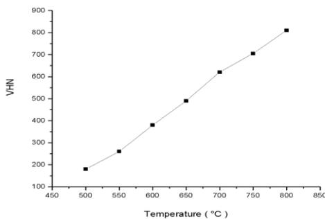
**Figure 4 :** Variation of VHN of the PZT thin films annealed at different temperatures
