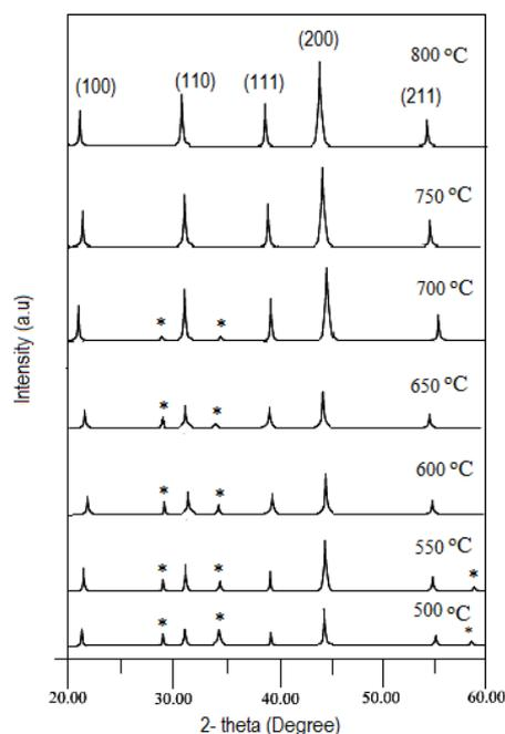
**Figure 1:** X- ray diffraction spectra of the PZT thin films annealed at different temperature 500 °C, 550 °C, 600 °C, 650 °C, 700 °C, 750 °C & 800 °C
