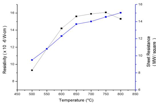
**Figure 2 :** Variation of Sheet Resistance and Resistivity with annealing temperature.
