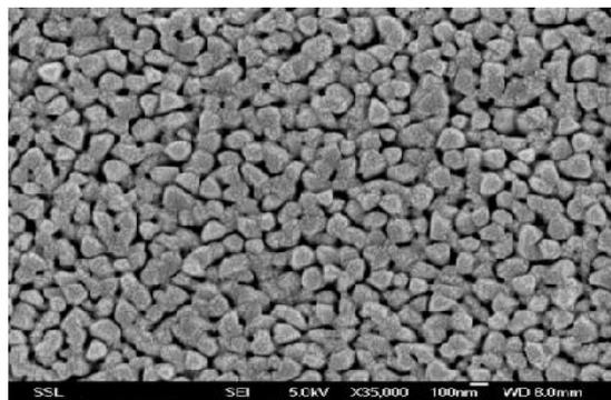
**Figure 8 :** SEM image of PZT thin film annealed at 800 °C
