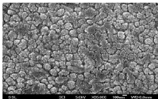
**Figure 6 :** SEM image of PZT thin film annealed at 600 °C
