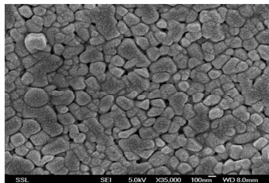
**Figure 7 :** SEM image of PZT thin film annealed at 700 °C
