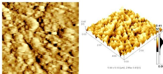
**Figure 5 :** 2D &3D AFM image of the PZT Thinfilm annealed at 800 °C
