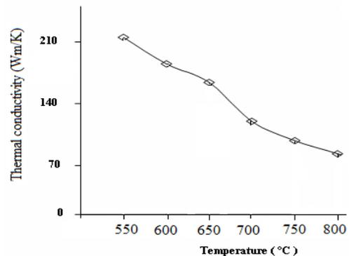
**Figure 3 :** Variation of Thermal Conductivity with annealing temperature.
