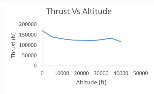
**Figure 5 :** Variation of Thrust at different Altitude
