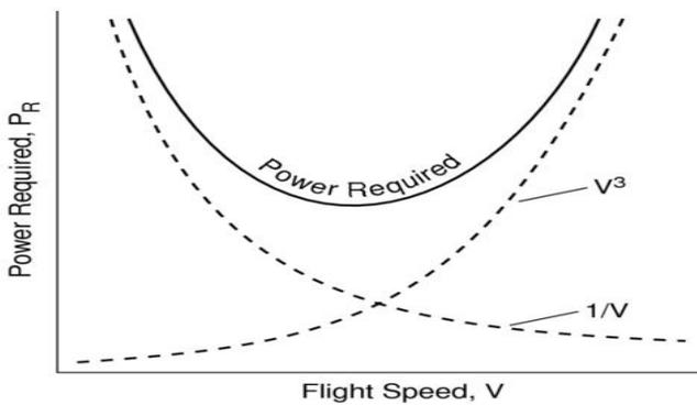
**Figure 6 :** Typical Power Required Curve for an Aircraft
