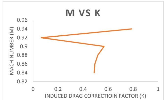
**Figure 4 :** Variation in induced drag correction factor at different Mach Number
