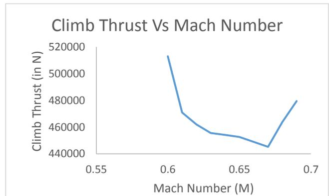
**Figure 8 :** Variation in climb Thrust at different Mach Number
